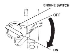
Figure 13. Engine ON/OFF Switch
